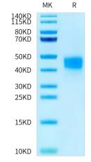
Human Fc gamma RIIIB (NA1) on Bis-Tris PAGE under reduced condition. The purity is greater than 95%.
