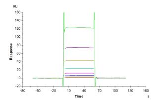
Human Fc gamma RIIIB (NA1), His Tag captured on CM5 Chip via anti-his antibody can bind Rituximab with an affinity constant of 8.55  $\mu$ M as determined in SPR assay (Biacore T200).
